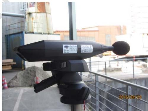
Calibrated noise measurement device
