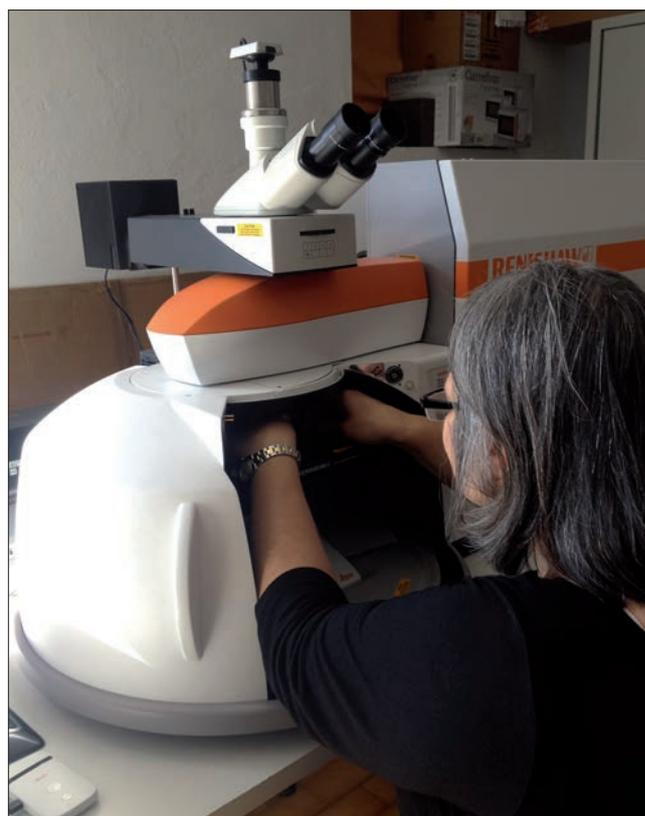
4. Operator at Raman spectroscopy.
