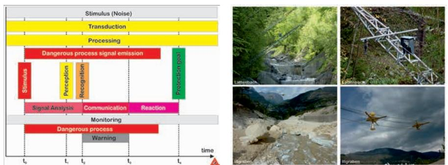
Figure 15: System of debris flow monitoring and warning technology, examples (Hübl & Mikoš, 2014)
