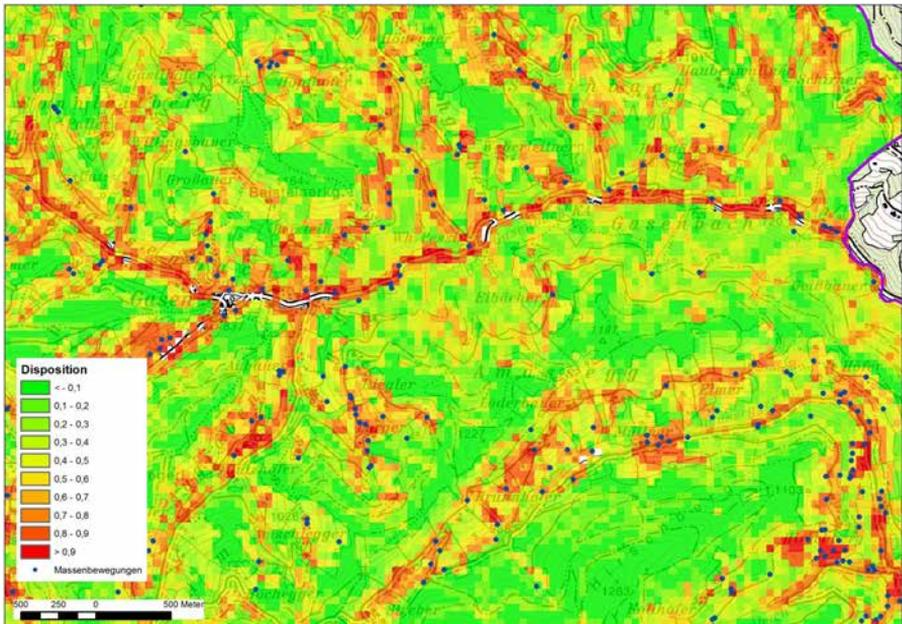
Figure 19: Modelling the disposition for shallow landslides in the area of Gasen and Haslau (Styria), based on documented events of the catastrophes in 2005 (© Geological Survey of Austria)
