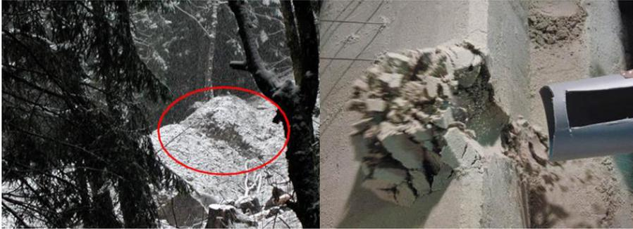
*Figure 28 left: documented impact in embankment with failure. right: model test with similar behaviour*
