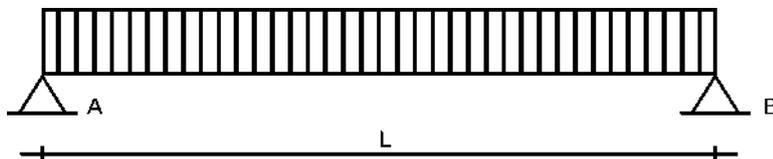
$$V_A = V_B = 795,19 \text{ Kg} \quad L = 1,50 \text{ m.}$$
