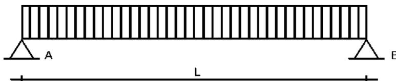
$$V_A = V_B = 1918,30 \text{ Kg} \quad L = 3,60 \text{ m.}$$
