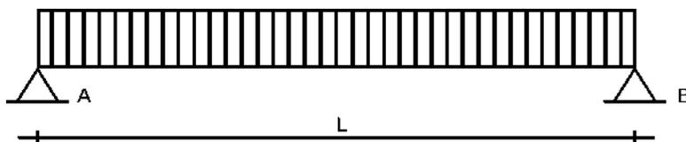
$$V_A = V_B = 1057,95 \text{ Kg} \quad L = 2,00 \text{ m.}$$
